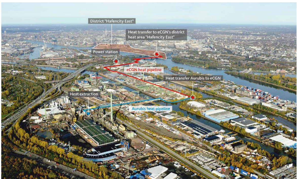
Fig. 1.8: District heating pipeline route
